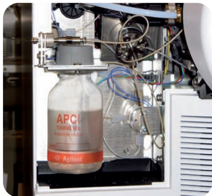
Built-in calibrant delivery system and premixed calibrants facilitate automated tuning.
