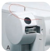
A Use the electrospray ionization (ESI) source to analyze large and small polar molecules.
