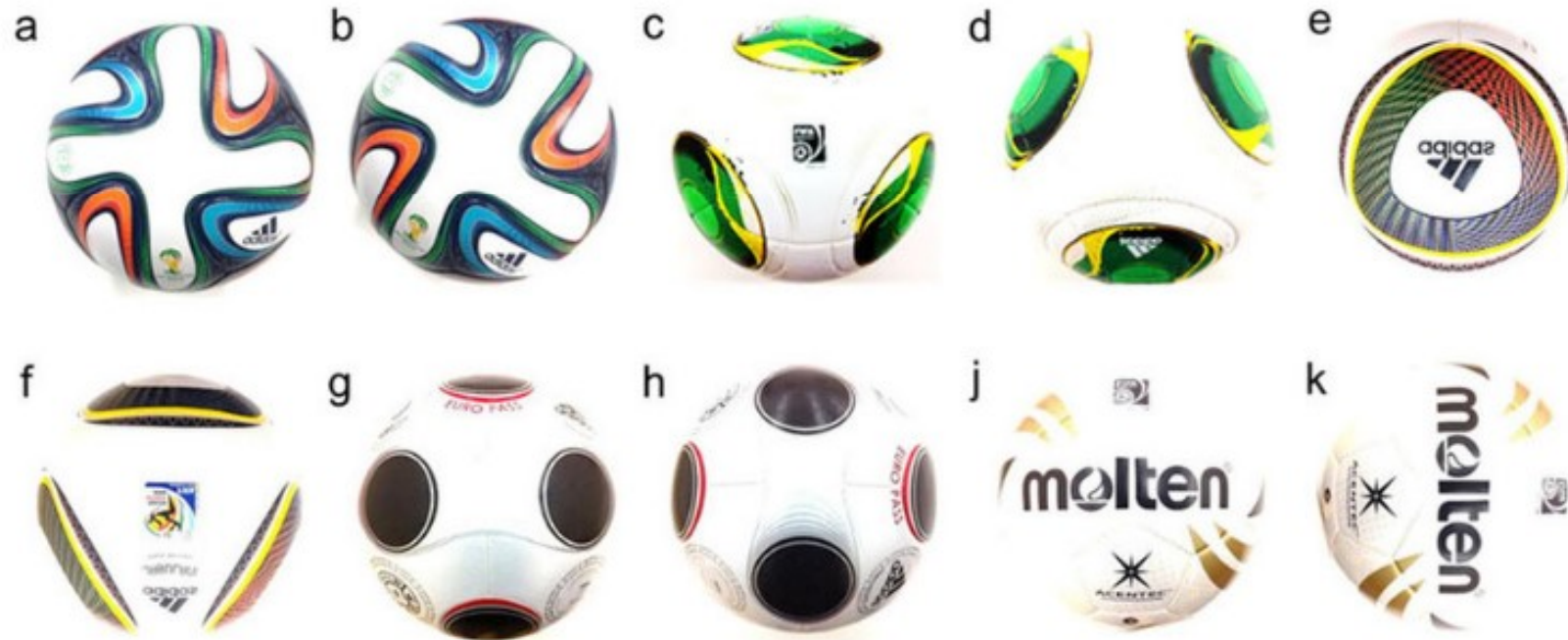
(a, b) Adidas Brazuca: small dimple and six panels, (c, d) Adidas Cafusa: small grip texture and 32 modified panels, (e, f) Adidas Jabulani: small ridges or protrusions and eight panels, (g, h) Adidas Teamgeist 2: small protuberances and 14 panels; (i, j) Molten Vantaggio (conventional soccer ball): smooth surface and 32 pentagonal and hexagonal panels. (Photo by S.H.).
