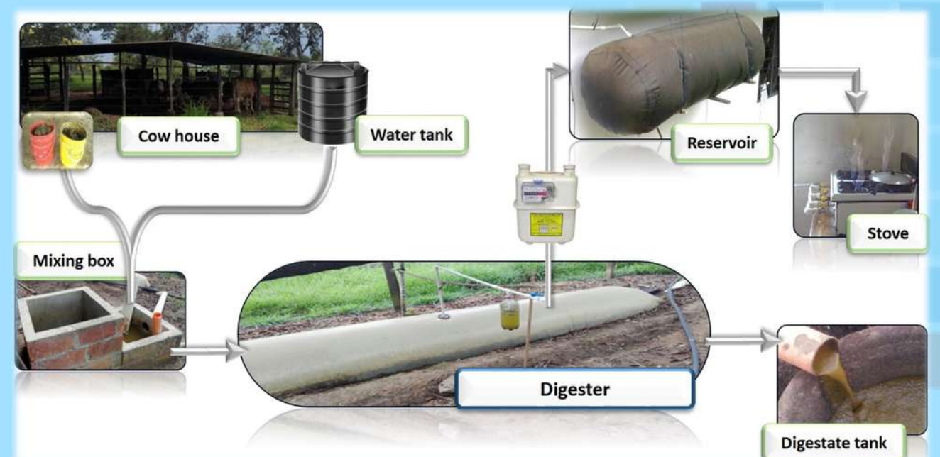
Fig. 2 Low-tech digester implemented in a small-scale farm
